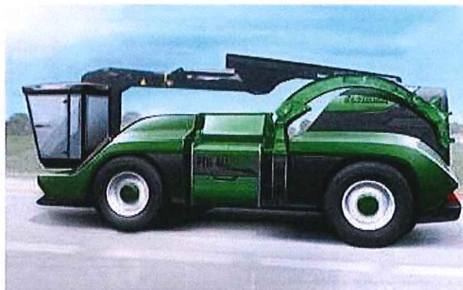
The drive is four-wheel and three different steering modes are possible
