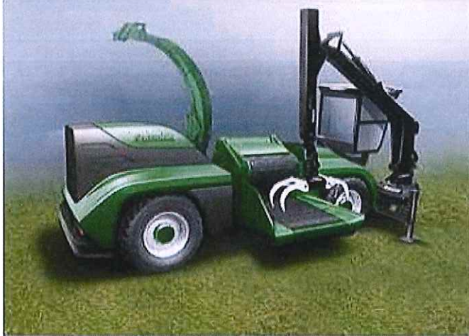
The inferior introduction roller has been changed with a longer feeding chain, able to transfer the material directly to the drum
