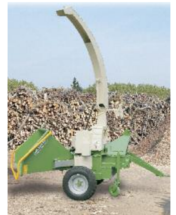
Chipping machine for chips heating system H 980/300 with extended output conveyor, equipped by hydraulic movements for deflector lifting, rotation and orientation
